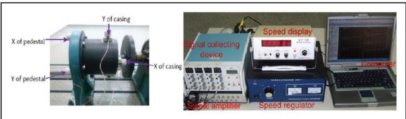
Figure 6. Distributions of vibration sensors (left) and data acquisition system (right).
