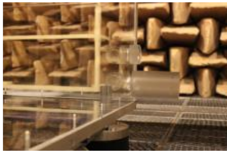
Figure 14 Experimental photo for the baffled open cavity coupled with a resonator in anechoic chamber.
