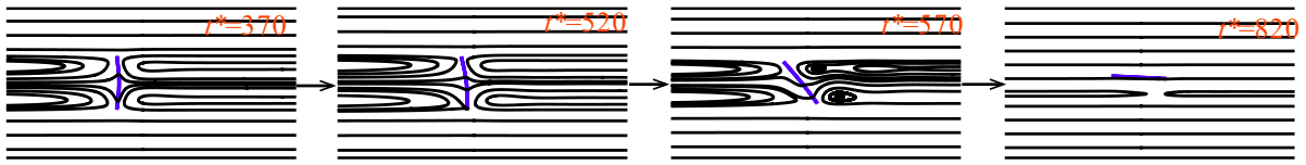
Fig. 15. Loss of the system stability and symmetry during the conveyance in the case of \theta_0 = 90^\circ (streamlines plotted based on the relative velocity between the flow and the fiber)
