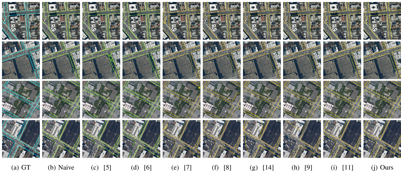
Fig. 6: Qualitative demonstrations. Each row shows an example. The first column is the ground truth (cyan lines); column (b) to (d) are segmentation-based baselines (green lines); column (e) to (i) are graph-based baselines and the last column shows the results of the new proposed imitation-learning-based baseline (orange lines for edges and yellow nodes for vertices). For better visualization, the lines are drawn in a thicker width while they are actually one-pixel width. The figure is best viewed in color. Please zoom in for details.
