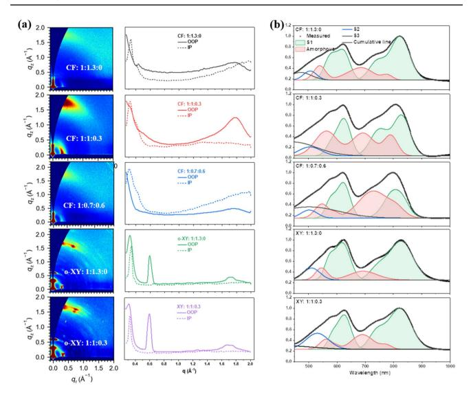
Fig. 3 Blend film morphology analysis: a 2D GIWAXS patterns and relative line-cuts. b UV-Vis spectra with gaussian fitting results
