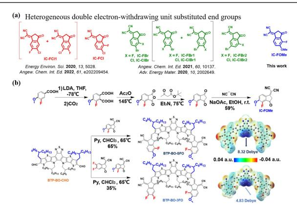
Fig. 1 a Design strategy of IC-FOMe; b Synthetic route and electrostatic potential of BTP-BO-3FO and BTP-BO-SFO
