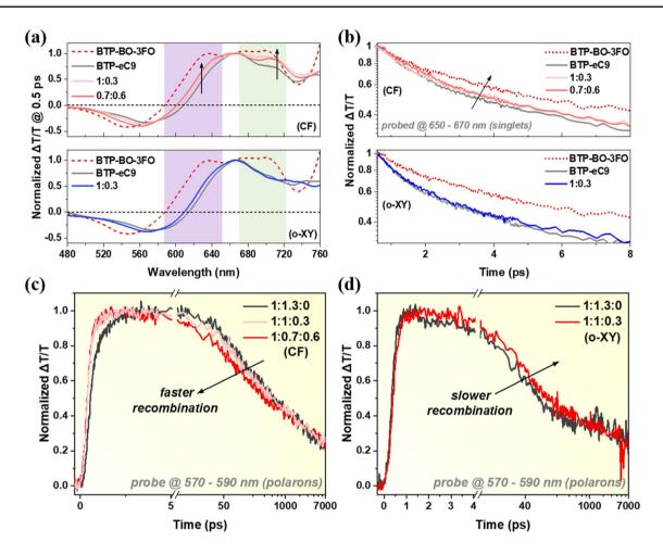
Fig. 5 a TAS spectra @ 0.5 ps after 800 nm pump laser for acceptor-only films. b Singlet excitons GSB signal decay kinetics of acceptor-only films. Exciton generation and recombination kinetics of c CF- and d o-XY-processed blend films
