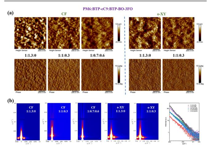
Fig. 4 a Blend AFM and b GISAXS
