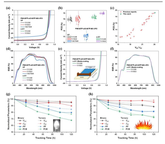
**Fig. 2** a *J-V* characteristics. **b** Normal distribution of PCEs. **c** A comparison of non-halogenated solvent processed OSCs. **d** EQE spectra. Blade-coating active layer from o-XY based binary and ternary solar cell performances: **e** *J-V* curves and **f** EQE spectra. **g** Light soaking stability of o-XY fabricated devices, and corresponding **h** thermal stability (80 °C)
