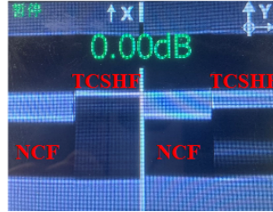
Fig. 4. The microscope image of the fusion splicing point between NCF and TCSHF.
