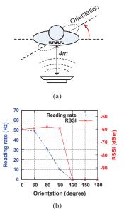
Figure 15. Reading rate and RSSI at different orientation.
