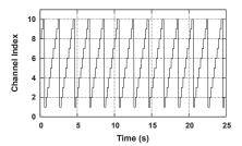
Figure 5. Channel hopping during the measurements.
