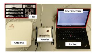
Figure 11. TagBreathe prototype system.
