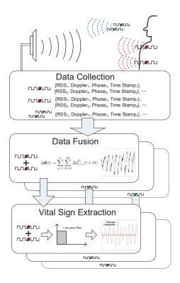
Figure 10. Illustration of TagBreathe workflow.
