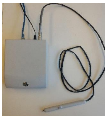
Fig.2. Ultrasound indentation device
