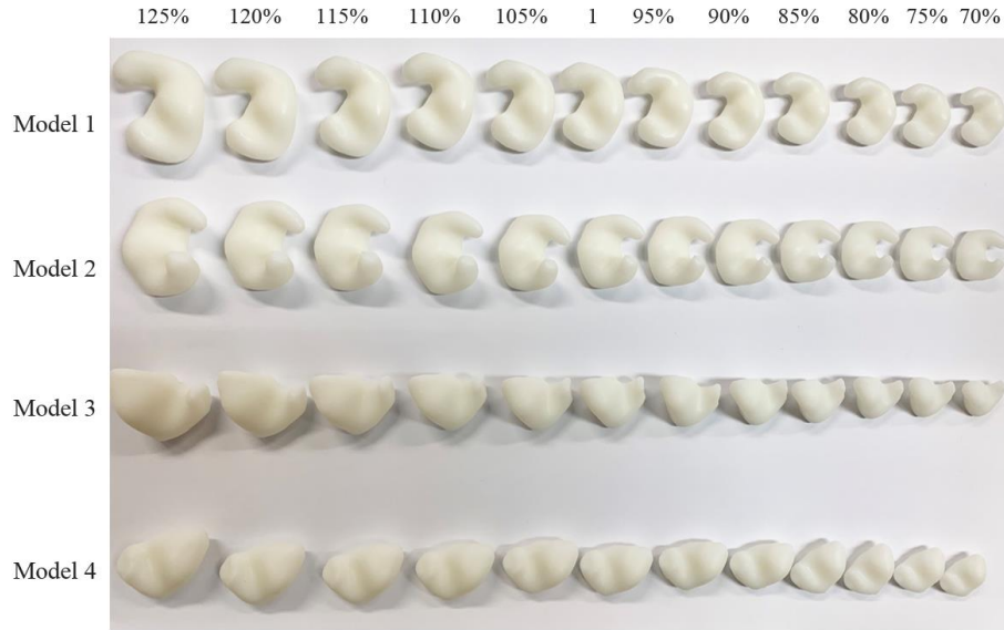
Fig. 1. Examples of prototypes: Model 1 : full-shell hearing aid without ear canal fitting; Model 2 : full-shell hearing aid with ear canal fitting; Model 3 : half-shell hearing aid with ear canal fitting; and Model 4 : half-shell hearing aid without ear canal fitting.
