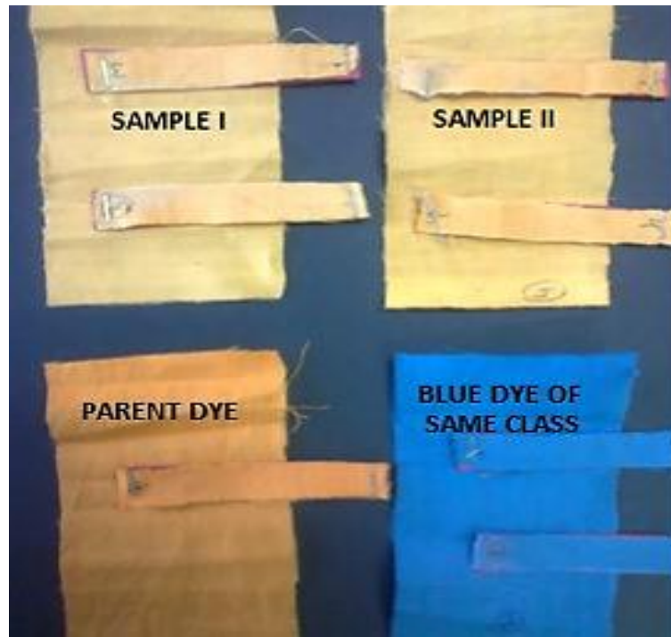
Figure 5: Light Fastness Test of the textile dyed with different nanoparticles. Sample I and Sample II present different textiles compared with the parental dye.
