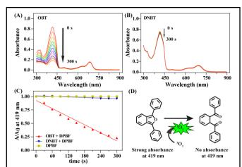
**Fig. 2**. The capability of the smart photosensitizer **OBT/DNBT** to generate ROS. UV-Vis absorption spectra of DPBF (100  $\mu$ M) and **OBT** ((A), 2  $\mu$ M) or **DNBT** ((B), 2  $\mu$ M) under irradiation with 660 nm laser at different time (0 s, 30 s, 60 s, 90 s, 120 s, 150 s, 180 s, 210 s, 240 s, 270 s, and 300 s); (C) Normalized DPBF degradation induced by different compounds under 660 nm light irradiation; (D) Schematics for the response of DPBF towards  $^1O_2$ .
