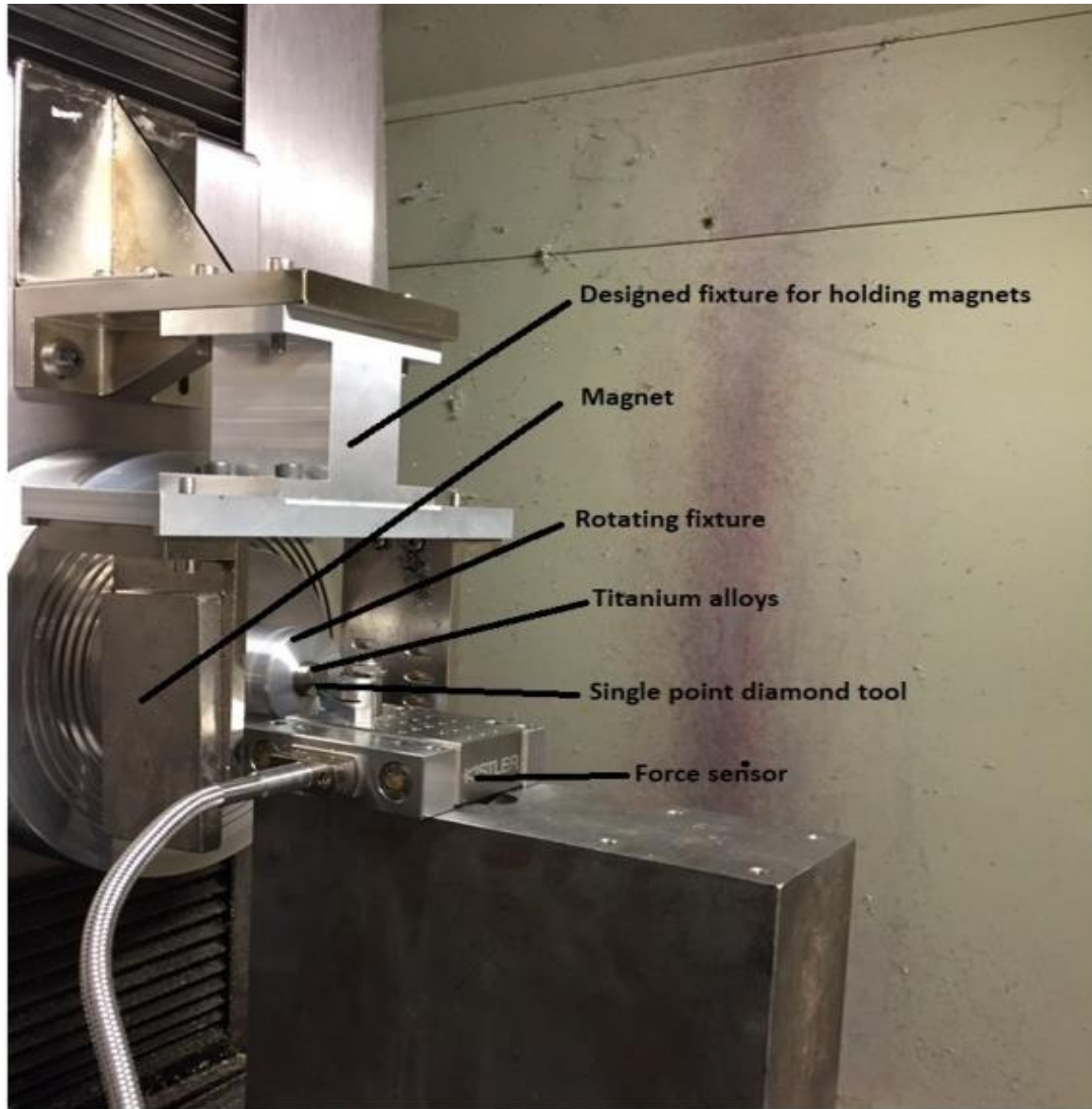
Figures 1. Experimental setup of SPDT under an eddy damping effect
