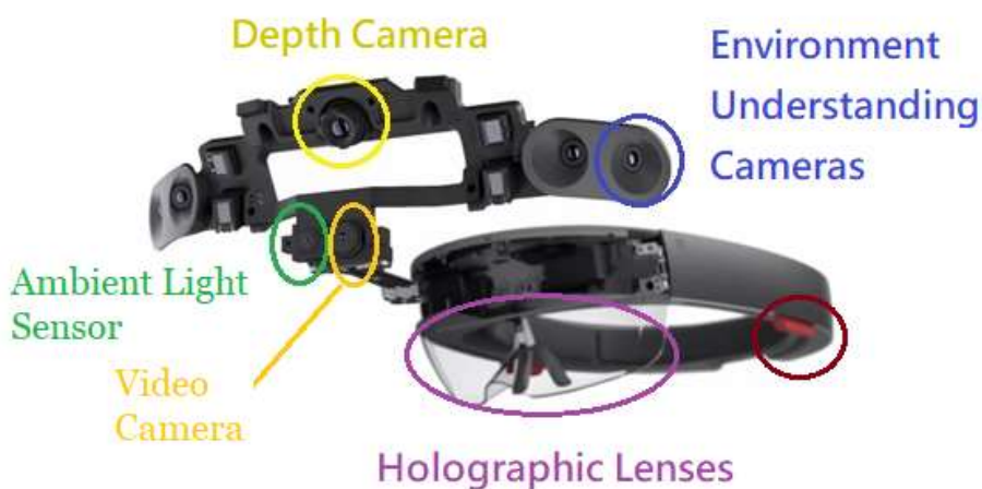
Figure 1 Hardware and configuration of the HoloLens
