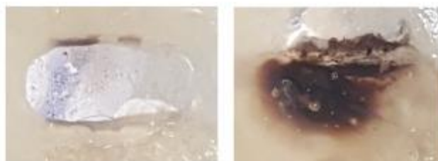
Fig. 1. Immersion dissolved oxygen sensor prototype made of 500 °C post-oxidized SCBD ZnO film . Left and right bottom: pictures of well and poorly protected immersion sensor taken after measurements in water.
