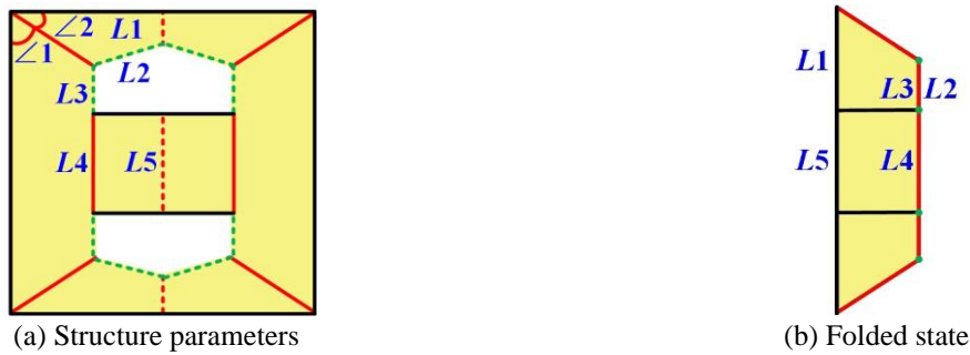
Fig. 13. Origami mechanism and its folded state
