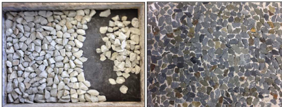
Fig. 2 – Test sample made with the Mosaic assembly method (Wang et al., 2018b).
