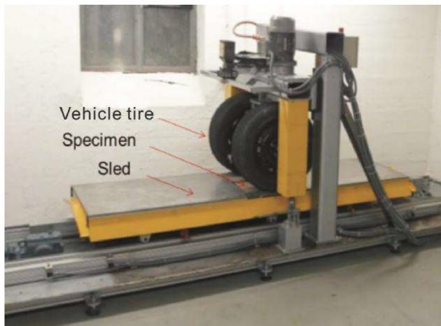
Fig. 3 – Aachen Polishing Machine (Wang et al., 2016; 2018a; 2018b).
