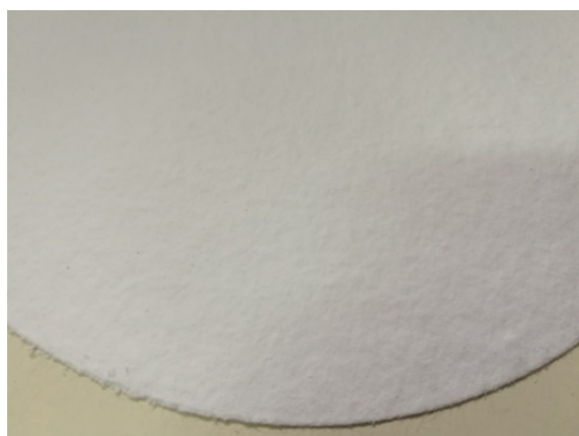
(a) Surface photo-Glass fiber HEPA media
