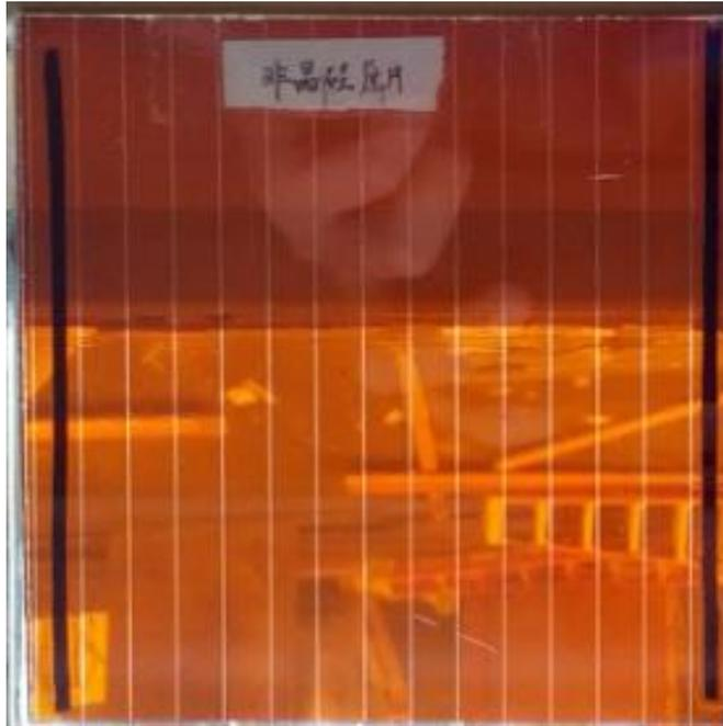
**Figure 2.** Photo of the semi-transparent a-Si sample used in this study
