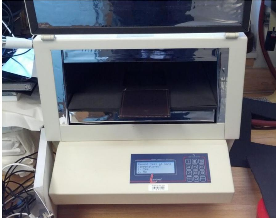
**Figure 6.** Measurement of the thermal conductivity of the PV sample
