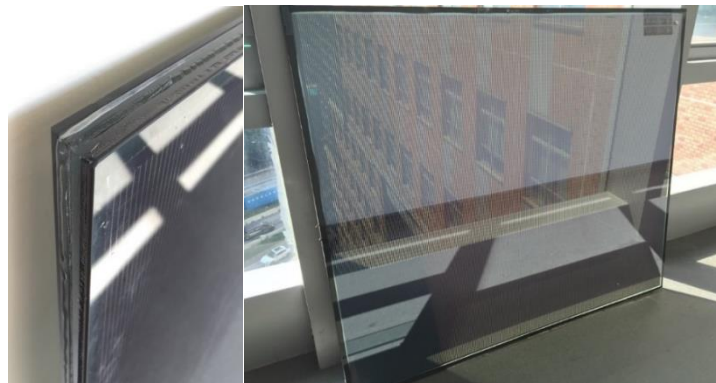
Fig 1. The cross-sectional view of vacuum PV insulated glass unit (Weilong Zhang, Lin Lu, & Xi Chen, 2016)
