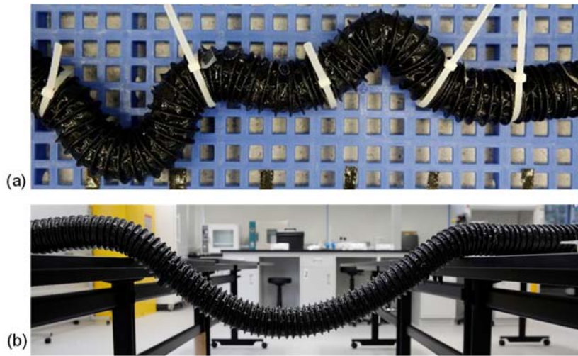
Figure 15. Photographic images of (a) a compressed flexible duct with multiple bends and (b) a flexible duct without support, leading to multiple bends.
