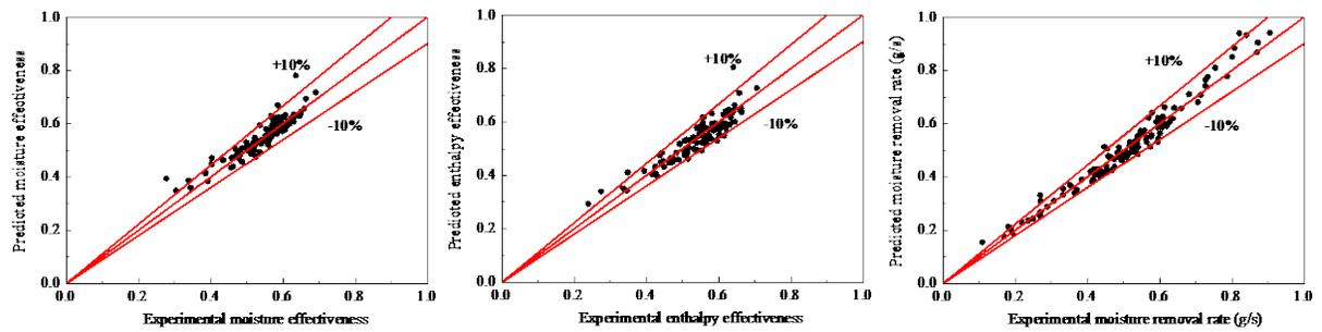
Fig.6. Comparison of predicted results and experiment results for the moisture effectiveness, the enthalpy effectiveness and the moisture removal rate.
