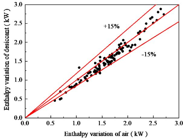
Fig.4. Energy balance analysis between air and desiccant solution.
