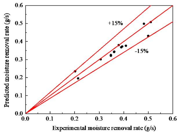
Fig.7. Comparison of predicted moisture removal rates and experiment results from Fumo and Goswami (2002).
