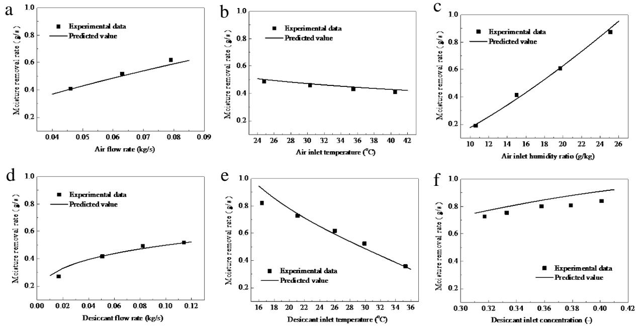
Fig.10. Influences of inlet parameters on the moisture removal rate.
