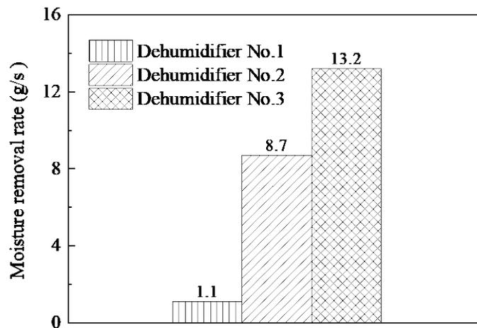
Fig.8. Moisture removal rates per unit packing volume for different dehumidifiers.
