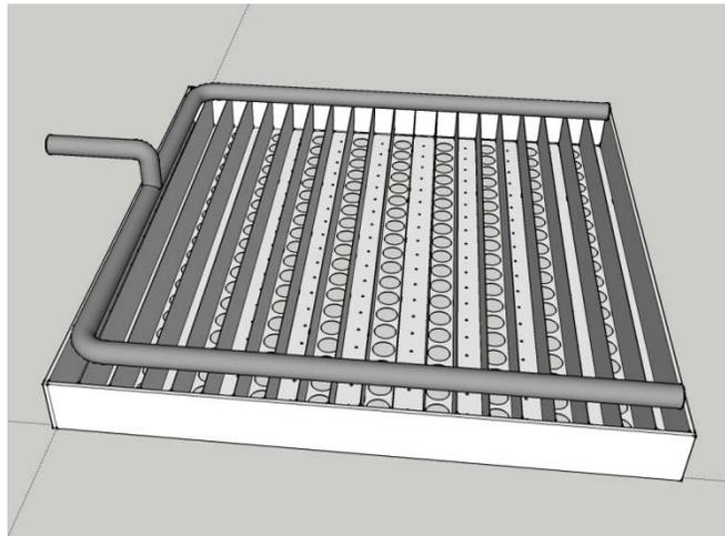
Fig.3. Porous plate distributor for desiccant solution.
