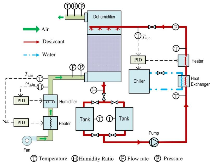
Fig.1. Schematic of experimental test rig.
