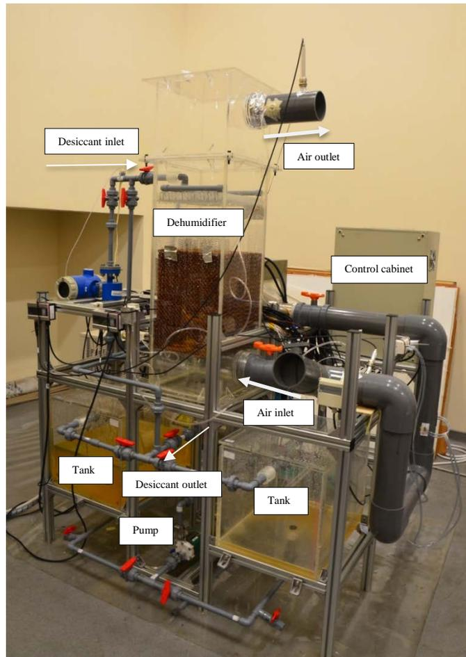
Fig.2. Photograph of experimental test rig.
