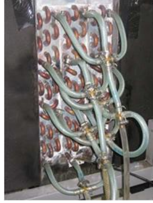
Fig. 1. The fin-tube type internally-cooled liquid desiccant dehumidifier [18]
