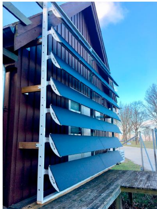
Fig. 29. Photograph of an outdoor PV blinds [92].
