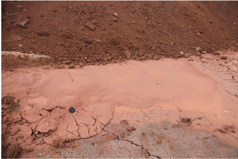
Fig. 6 Fully liquefied soil in sliding surface.
