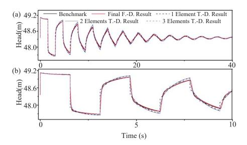
**Fig. 9** Results comparison of transient traces using calibrated K-V elements from the Time-Domain (T.-D.) and Frequency-Domain (F.-D.) methods (a) overview of the whole simulation traces; (b) enlarged part of the first 2 wave cycles.
