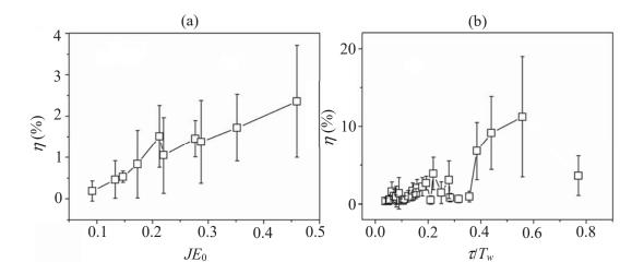
**Fig. 12** Influence of pipe material properties on the developed FDTBM: (a) ratio of the viscoelastic modulus and elastic modulus; (b) ratio of the retardation time scale and wave time scale
