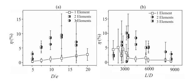
**Fig. 11** Influence of pipe scale parameters on the developed FDTBM: (a) diameter-thickness ratio; (b) length-diameter ratio
