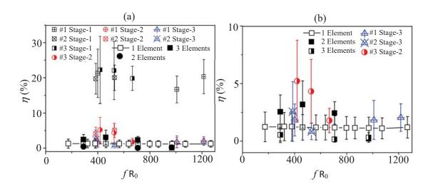
Fig. 10 Influence of unsteady friction on the application of the developed FDTBM: (a) the evolution of the multistage calibration process for the numerical and experimental tests; (b) final results of numerical and experimental applications for different tests and systems
