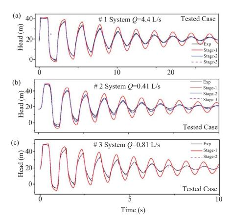
**Fig. 4** Calibrated and measured results of transient pressure traces: (a) #1 system; (b) #2 system; (c) #3 system
