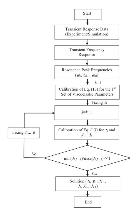
Fig. 2 Overall procedure for the multistage FDTBM
