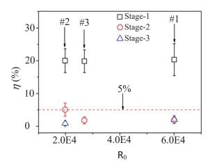
**Fig. 5** Stage-by-stage evolution of the errors in transient pressure amplitudes for the multistage calibration procedure of FDTBM
