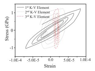
Fig. 6 Stress-and-strain curve of the calibrated three K-V elements in the test #1 system
