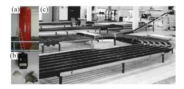
**Fig. 3** Experimental facilities at the University of Perugia, Italy: (a) pressurized air vessel; (b) pressure transducer; (c) HDPE pipes
