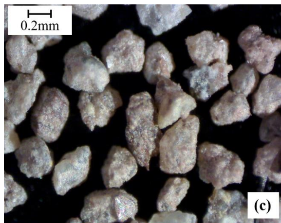
Figure 2. The photos of typical soil particles of fill material in the size ranges of (a) 10-20 mm; (b) 0.3-2 mm; (c) 0.212-0.3 mm; (d) 0.063-0.212 mm
