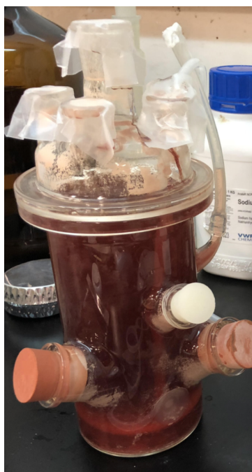
Fig. 3 Lab-scale reactor for the recovery reaction by metal-TCPP
