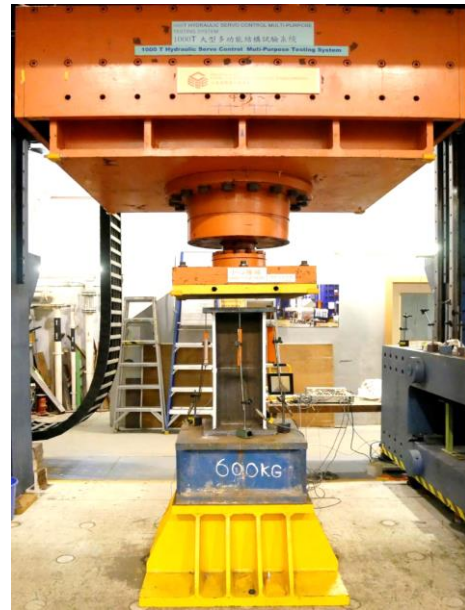
b) 1000 tons Hydraulic Servo Control Testing System
