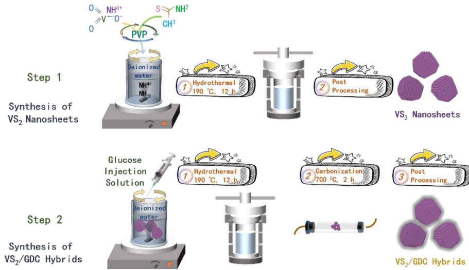
Fig. 1. Schematic illustration of the growth of VS 2 nanosheets and VS 2 /GDC hybrids.
