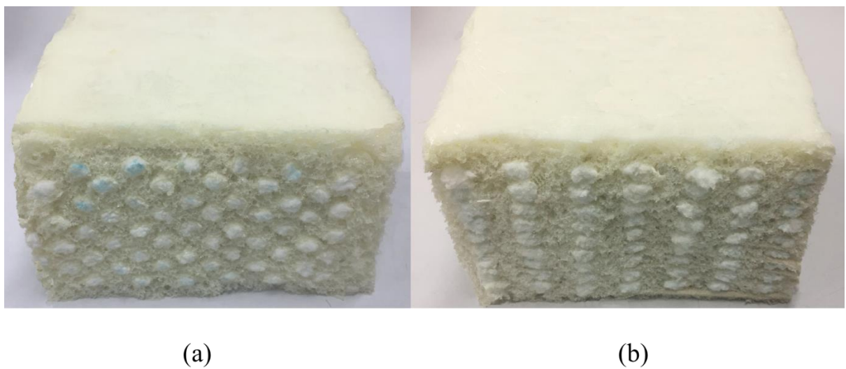
Fig. 4 3D textile composites fabricated: (a) auxetic; (b) non-auxetic.
