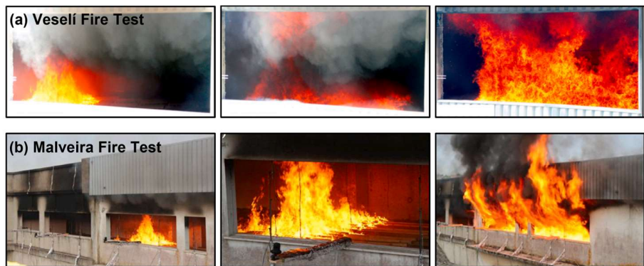
122 123 Fig. 2 Typical photos of travelling fires: (a) Veseli Fire Test [13] and (b) Malveira Fire Test [15].
