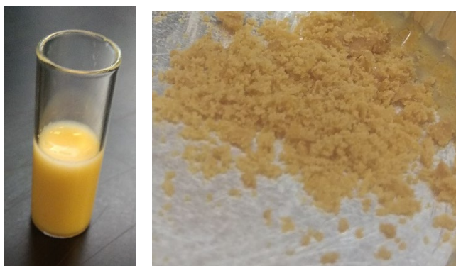
Figure S4. Appearance of NEPCM dispersion in water and in dried powder.
