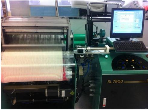
Figure 2. Optical fiber integrated fabric processing on a weaving machine
