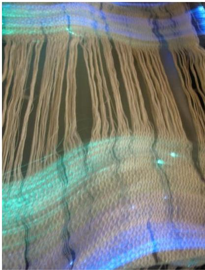
Figure 3. Photonic fabric swatch
