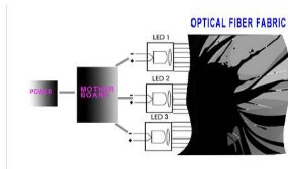
Figure 5. Schematic diagram of the POFF system
