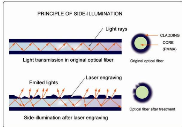
Figure 4. Principle of side-illumination by laser-engraving
