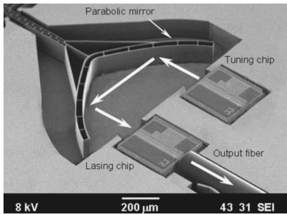
FIG. 2. Scanning electron micrograph of the MEMS coupled-cavity laser formed by integrating a Fabry-Pérot chip (as the lasing chip), a gain chip (as the tuning chip) and an output fiber with a deep-etched parabolic mirror.
