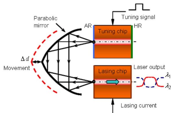
FIG. 1. (Color online) Design of the tunable coupled-cavity laser constructed by the MEMS technology.
