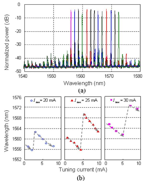
FIG. 4. (Color online) Wavelength tuning characteristics of the MEMS coupled-cavity laser. (a) Superimposed spectra at different tuning currents for a fixed lasing current of 25 mA and (b) measured output wavelengths as a function of the tuning current under different levels of lasing currents.
