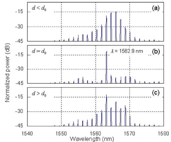
FIG. 3. (Color online) Output spectra of the MEMS coupled-cavity laser at different gaps. (a) Multimode emission at  $d < d_0$ , (b) single-mode output at the optimal state of  $d = d_0$ , and (c) multimode emission at  $d > d_0$ .
