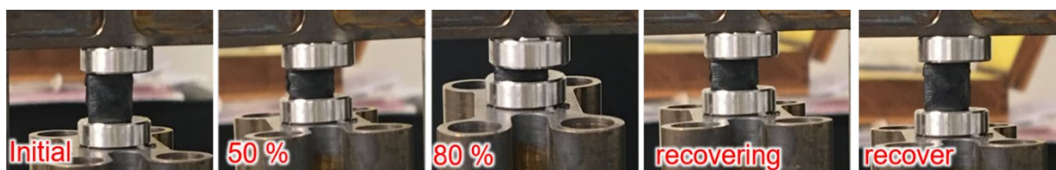
Figure S5. Optical images showing the reversible compressions of the crosslinked graphene-based aerogels with a strain of 80%.
