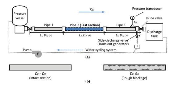
**Fig. 5.** Experimental test system: (a) sketch of test system configuration; (b) inserted sections for the two test cases (intact and rough blockage sections).
