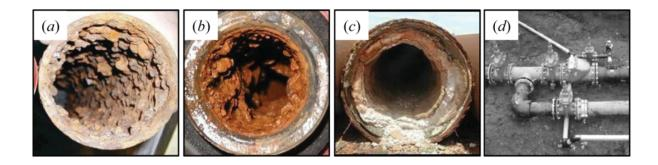
**Fig. 1.** Disorders of pipe diameters (roughness and blockages) in water pipelines due to different factors: (a) corrosion; (b) bio-film; (c) deposition; (d) complex connection.
