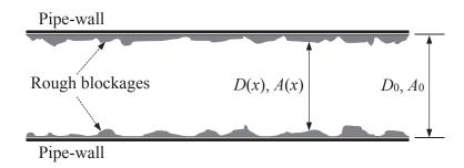
Fig. 2. Sketch of rough blockage configuration in a water pipe section.
