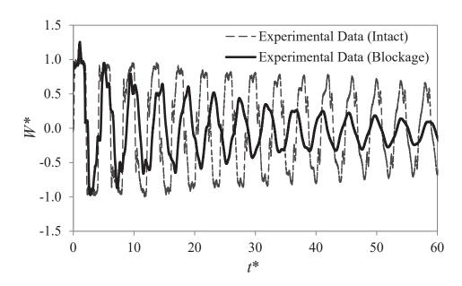
**Fig. 6.** Time-domain measurement of transient waves for two test cases  $(0\sim60\ L/a)$ .
