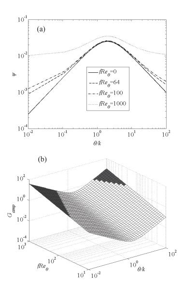
Fig. 3. Effects of pipe wall roughness and blockage on transient wave envelope attention: (a): dimensionless envelope attenuation coefficient ( $\psi$ ); (b): relative importance ( $G_{amp}$ ) with the black-filled region for  $G_{amp} > 1$ .
