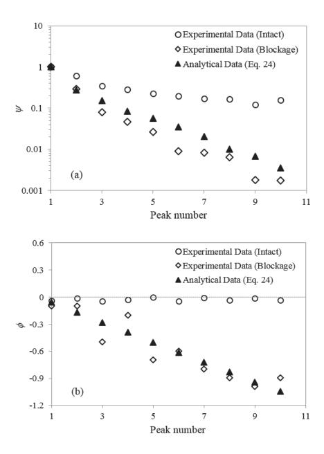
**Fig. 7.** Frequency-domain results of two test cases (with first 10 peaks) for: (a): peak amplitude attenuation; (b): peak frequency shift (phase change).
