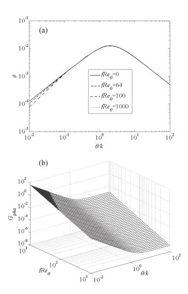
Fig. 4. Effects of pipe wall roughness and blockage on transient wave phase change: (a): dimensionless phase change coefficient  $(\phi)$ ; (b): relative importance  $(G_{pha})$  with the black-filled region for  $G_{pha} > 1$ .
