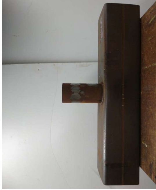
Fig. 23. Chord side wall failure mode (S) comparison between test and FE RHS-RHS T-joint
