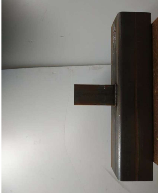
Fig. 21. Chord face failure mode (F) comparison between test and FE RHS-RHS T-joint
