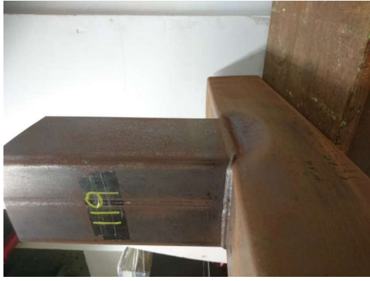
Fig. 23. Chord side wall failure mode (S) comparison between test and FE RHS-RHS T-joint
