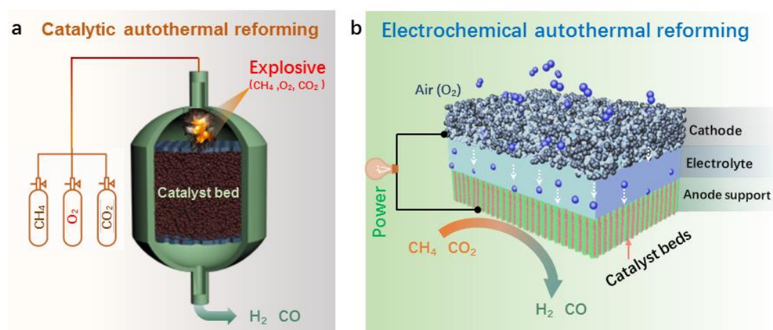
Fig. 1. Schematic comparison of (a) conventional autothermal reforming of methane within catalyst bed reactors and (b) electrochemical autothermal reforming of methane over SOFCs.
