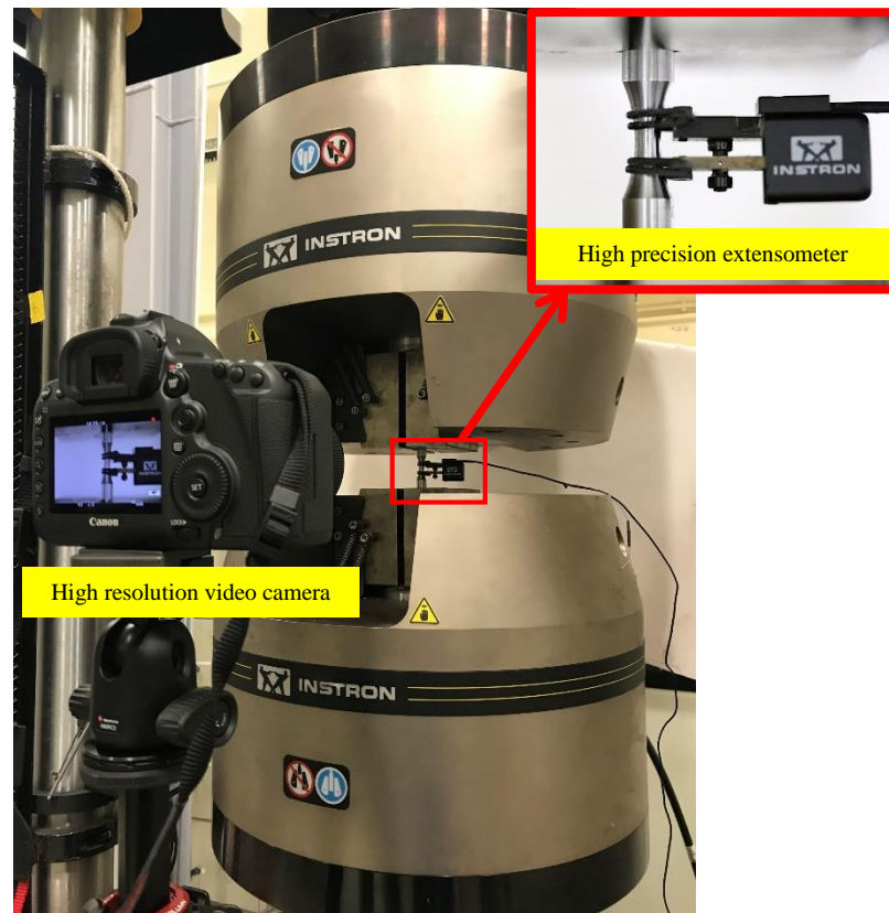
Figure 5 Test set-up for both monotonic and cyclic tests
