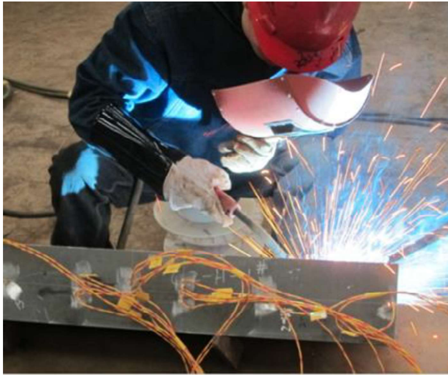
Figure 4 Welding of an I section – GMAW
