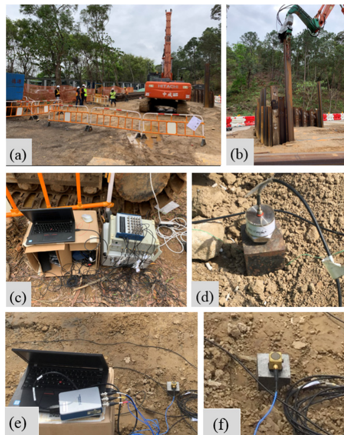
Figure 13. Photos of field validation test setup. (a) The construction site; (b) the vibratory sheet pile driving work in progress; (c) the first set of data acquisition systems integrated with (d) the single-axis accelerometers; (e) the second set of data acquisition system integrated with (f) the triaxial accelerometer.
