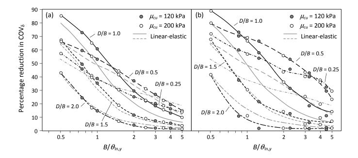
FIG. 5. Reduction in  $COV_{\delta}$  for strip footings on  $c_u$  soil (FS=2.0) with (a)  $COV_{cu}=0.15$ ; and (b)  $COV_{cu}=0.4$
