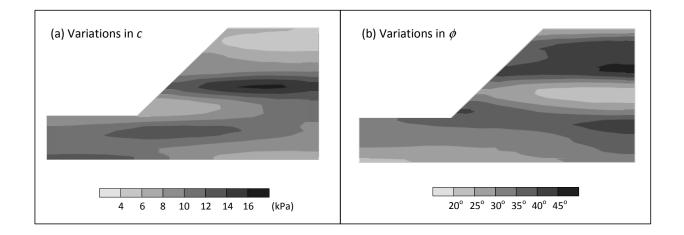
FIG. 2. Typical realizations of random fields of cohesion and friction angle, with cross-correlation coefficient of  $-0.5\,$
