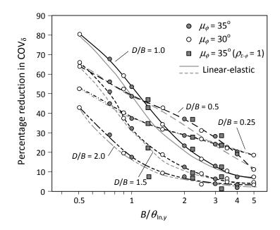
FIG. 8. Reduction in COV $_{\delta}$  for strip footings on  $\phi$  soil (FS=2.0)
