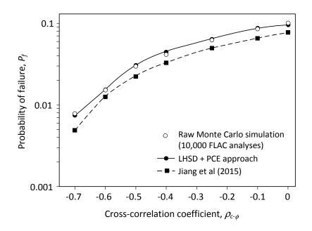
FIG. 3. Probability of failure in slope stability analyses
