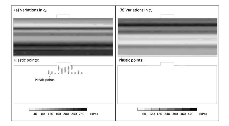
FIG. 6. Realizations with  $\mu_{cu}$  =200 kPa, COV $_{cu}$  =0.4 and  $\theta_{\ln,y}$  =0.4 m but different distributions with depth
