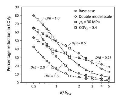
FIG. 4. Reduction in  $\text{COV}_{\delta}$  for strip footings on linear-elastic soil
