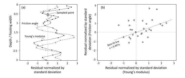
FIG. 7. (a) Residuals for simulated profiles of Young's modulus and friction angle; (b) Correlations between the normalized residuals
