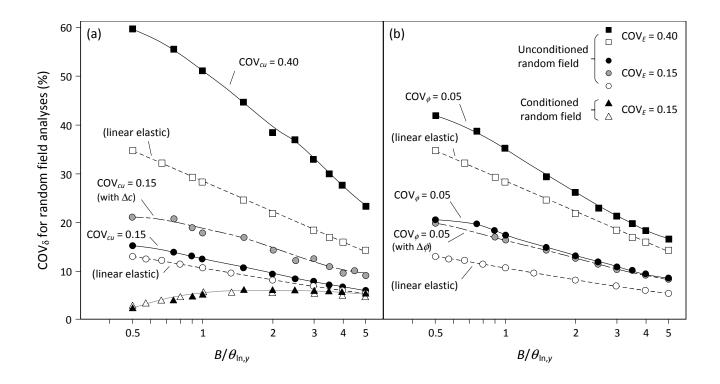
FIG. 9. COV $_{\delta}$  for strip footings on (a)  $c_u$  soils and (b)  $\phi$  soils
