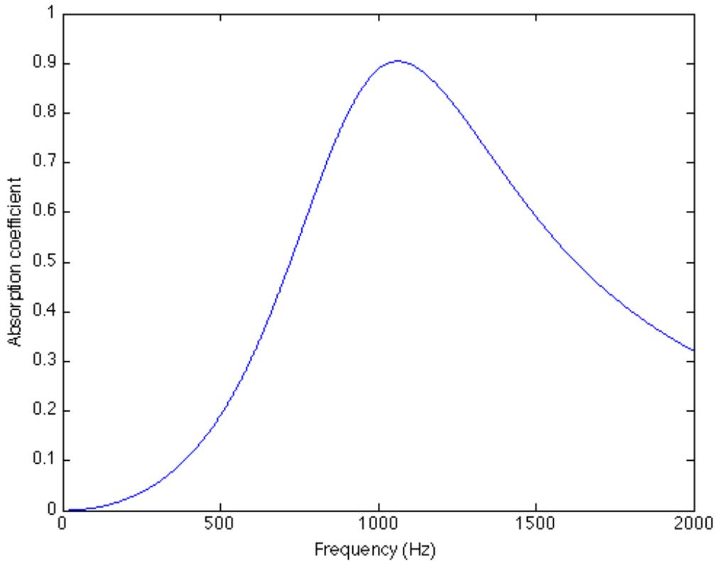
Figure 3 Sound absorption coefficient curve for the MPP having a backing air layer of depth 30mm.
