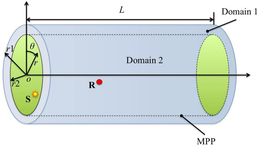
Figure 1 Diagram for the MPP lined on the inner wall of a cylindrical acoustic domain, a uniform air space of depth  $r_1-r_2$  is left behind the MPP.
