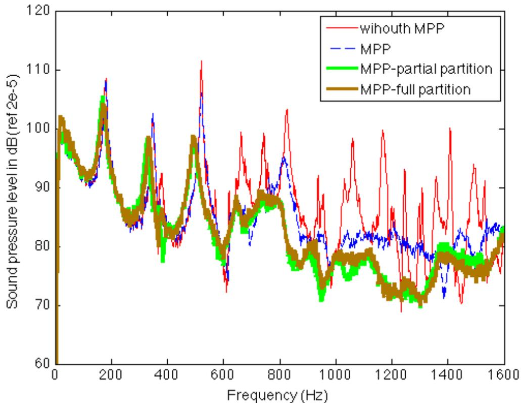
Figure 6 Measured interior sound pressure level: Symmetric excitation.
