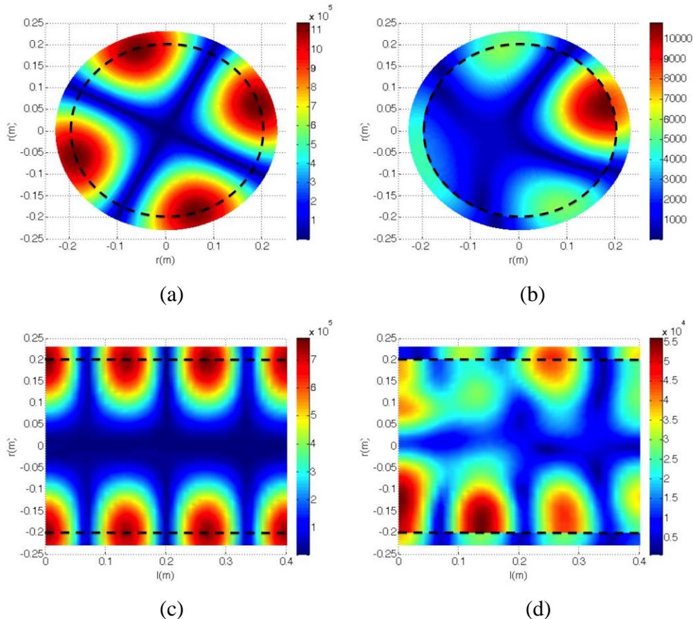
Figure 4. Cross-sectional view of the sound pressure distribution at different frequencies: (a) 942Hz, plane normal to the axis  $l = 0.3$ m; (b) 1046Hz, plane normal to the axis at  $l = 0.3$ m; (c) 1536Hz, plane parallel and passing through the axis; (d) 1514Hz, plane parallel and passing through the axis. (dash line: MPP)
