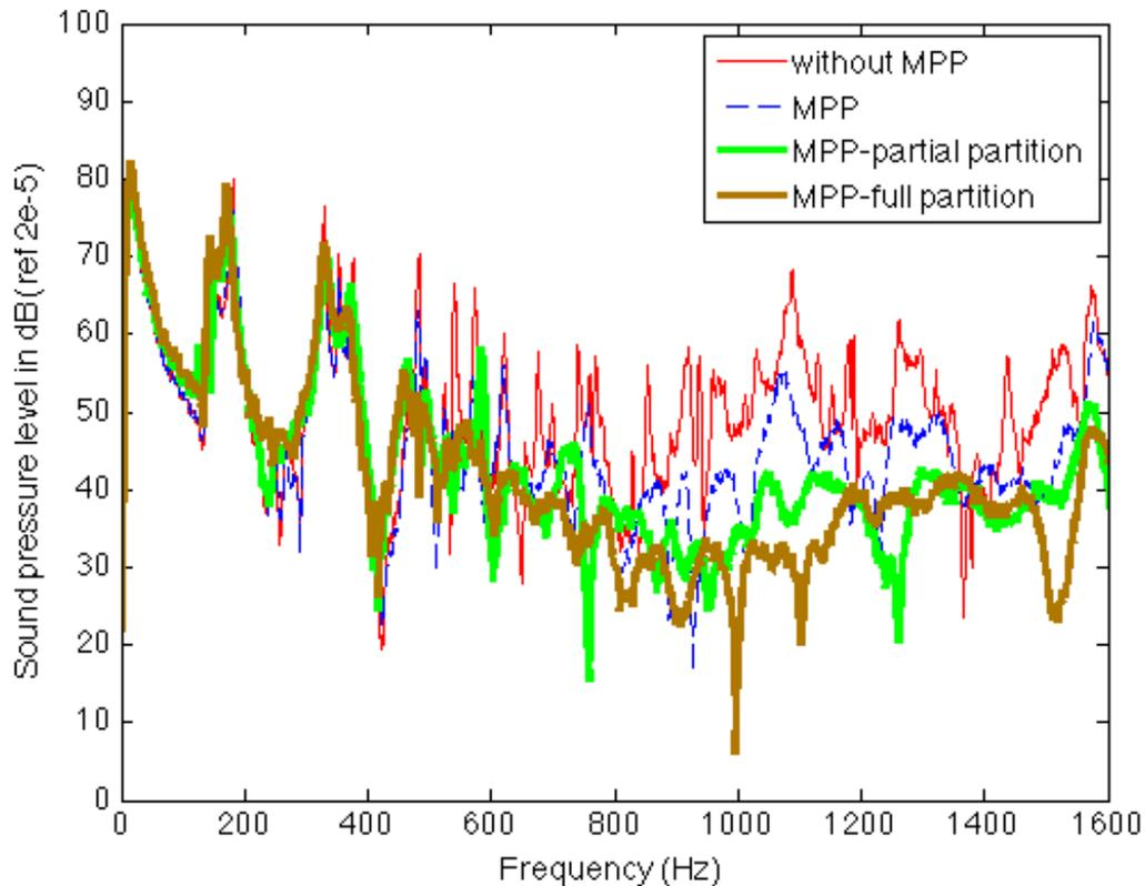
Figure 8 Measured interior sound pressure level: Non-symmetric excitation.
