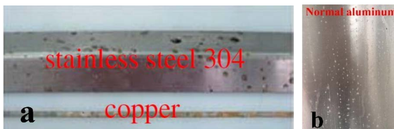
Fig. 1. Corrosion phenomenon of liquid desiccant on metals [18, 19].
