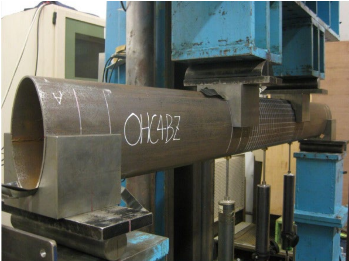
(b) Experimental setup of four-point bending test
