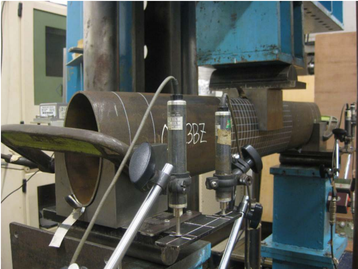
(b) Experimental setup of three-point bending test
