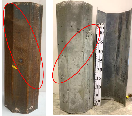
Fig. 6. Typical failure modes (Specimen O75x3-90).
