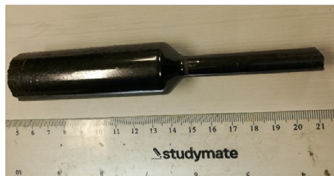
Figure 2. As-grown boule of Mn-modified PIN-PMN-PT single crystal.
