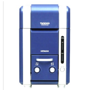
(b) Scanning electron microscope, Hitachi TM3000
