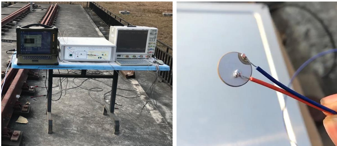
225 Fig. 4. Online diagnosis system and the PZT wafers used to construct sensor network 226
