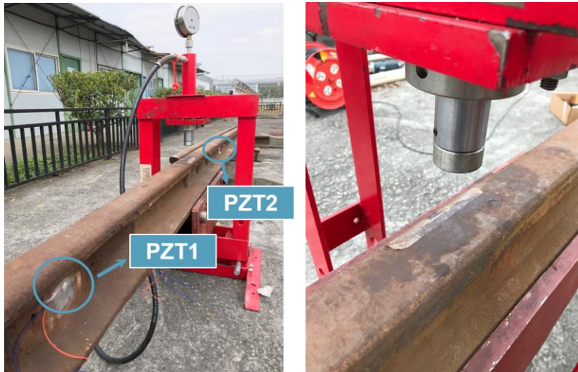
300 Fig. 8. The hydraulic press used to exert load on the rail and the sensor network on the web 301 of the rail
