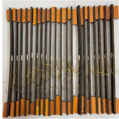
Fig. 24 Deformed strips from CF2-145 × 6 after sectioning process
